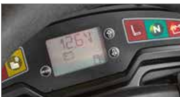
The LCD display provides quick and intuitive consultation of the main information of the garden tractor, including working hours, battery voltage, and fuel level.
