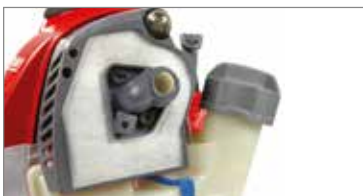
Filter support with anti-backflow element (Emak patent): prevents the filter from becoming fouled by fuel and guarantees longer operation between filter maintenance procedures.
