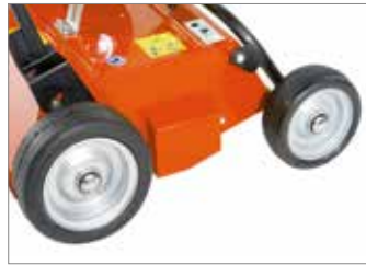
Metal wheels with ball bearings.
