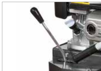
Speed selection control lever.
