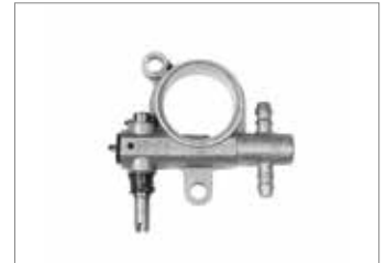
Adjustable aluminium oil pump: facilitates the operator's job by allowing the oil feed to be adjusted to suit the workload on the machine and the bar/chain combination. Zero oil flow with the engine at idling speed ensures lower consumption and reduced environmental impact.
