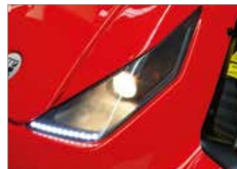
Halogen headlights and LED worklights ensure a good view of the cutting area, even in low light conditions.
