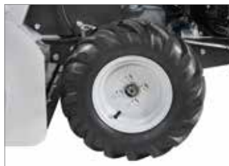
Generously sized tyred wheels (4.00-8") to ensure excellent grip on the ground.
