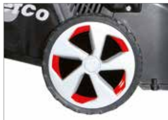
Large size IMPACT series wheels (Ø 280 mm rear and Ø 200 mm front) with shielded ball bearings: guarantee of smoother movement and optimal traction on all types of terrain.
